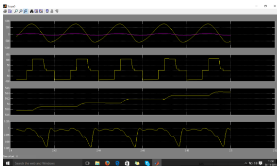
Fig 3: in phase voltage currents and transformer voltage and load current and power factor of proposed converter
