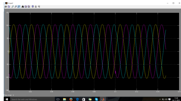
Fig 7: voltage after removing the unbalanced voltage sag
