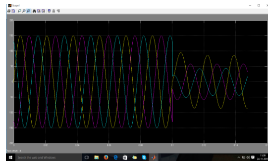
Fig 6: unbalanced sag of system
