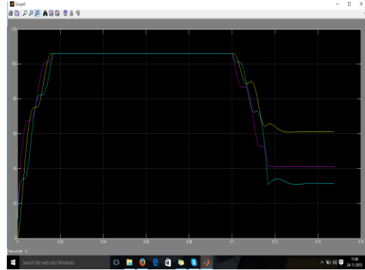
Fig 5: rms voltages under sag
